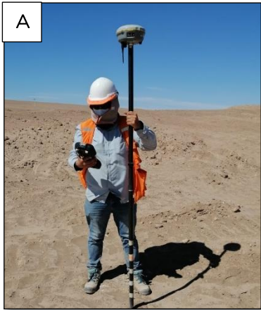
Figure 8-1. A) Drilling Point Marking B) Drill Rig Positioning C) RC Drilling D) RC Samples at Platform
